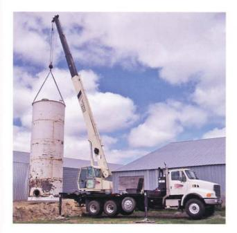
**Cranes** - Dan Poland Machine also offers a 30 Ton National Crane with 110' of hydraulic stick and an addition Jib of 44'. The crane can also be equipped with one or two man baskets. Rigging and moving is also available.
